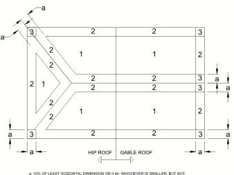
a: 10% OF LEAST HOIZONTAL DIMENSION OR 0.4h, WHICHEVER IS SMALLER, BUT NOT LESS THAN EITHER 4% OF LEAST HORIZONTAL DIMENSION OR 3FT (0.9M). OR AS DETERMINED BY DESIGN OR OTHER APPLICABLE CODE.
